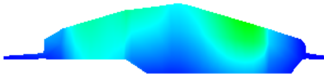
Figure 4-33. Predicted equivalence ratio distribution a) 300 Bar injection pressure at -3 deg ATDC b) 500 Bar injection pressure at -5 deg ATDC
